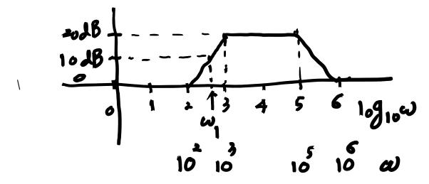
[5].(20 points) The following figure show a Bode plot of a band-pass filter.
